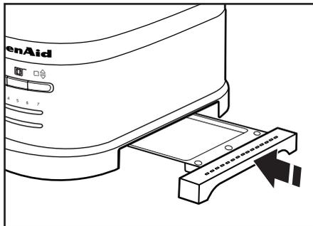
Wipe toaster with a soft, damp cotton cloth. Do not use paper towels, abrasive cleansers or liquid cleaning products. Do not immerse toaster in water.
