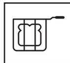
2. Insert the Sandwich Rack into the toaster slot, with your sandwich inside, as shown. The toaster will automatically lower the Sandwich Rack and start toasting.
